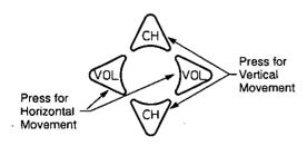
7. Align the horizontal and vertical lines with the frame mechanical reference marks. Press or on Remote Control for moving the vertical line and and or for moving the horizontal line.
