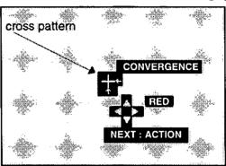
9. Align the Red Cross with the white cross pattern at the center of the screen. Press or on the Remote Control for horizontal movement and or of for vertical movement.
